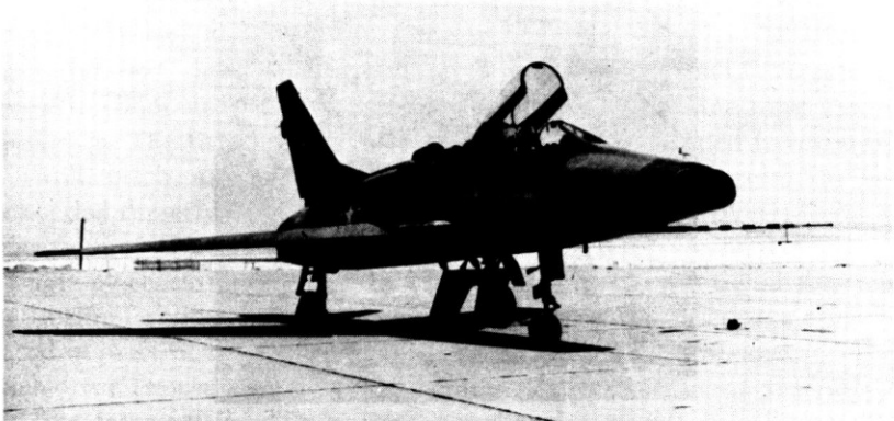
Fig. 3. F-100C variable-stability airplane.
